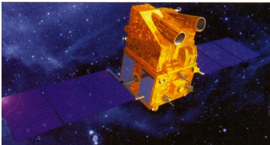
*Figure 1: Cartosat-1 = IRS-P5; stereo imaging with two cameras; 26° forward; 5° after*
