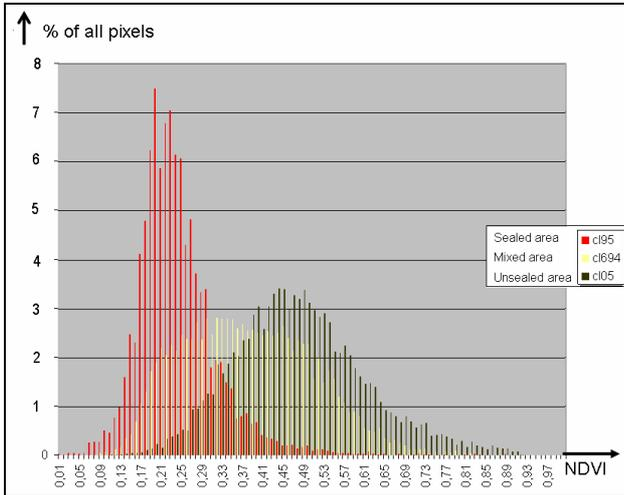
Figure 6: **Pixel level.** Two histograms for 'pure pixels' and one for mixed pixels; x-axis=NDVI value from SPOT5. Pure sealed area in red (values in degraded IKONOS ranging from 95-100), Pure unsealed area in black (values 0-5). Mixed pixels in yellow (values 6- 94).
