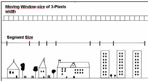
Figure 2. (after Blümel, 2000). Moving window filtering has a fixed size (here 3\*3). Segment-size is varying with more than 30 pixels per object primitive.
