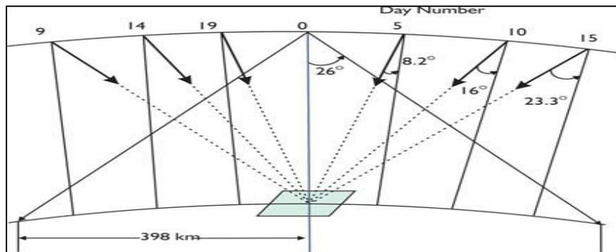
**Figure 8.30 Steerability of LISS-IV camera**
