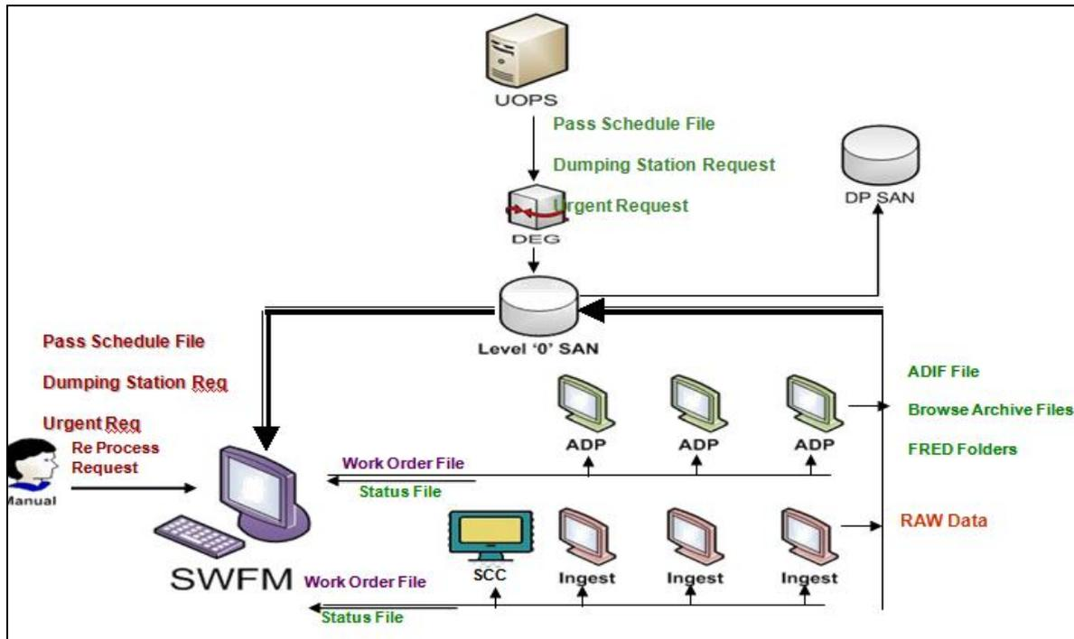
Fig. 6.2 Overview of Station Work Flow Manager
