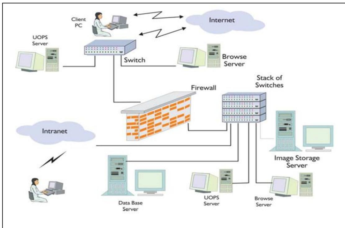
Fig. 8.1 Block diagram of User Order Processing System
