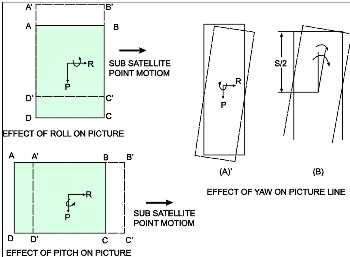
Figure 3.12 Effect of attitude errors on image
