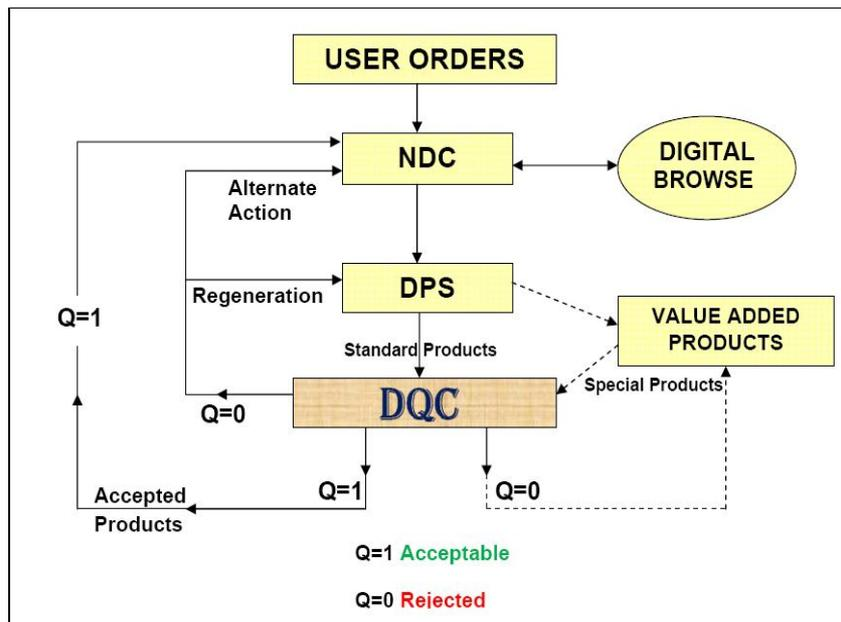
Fig. 7.3 Flow Chart for Generation of Digital products
