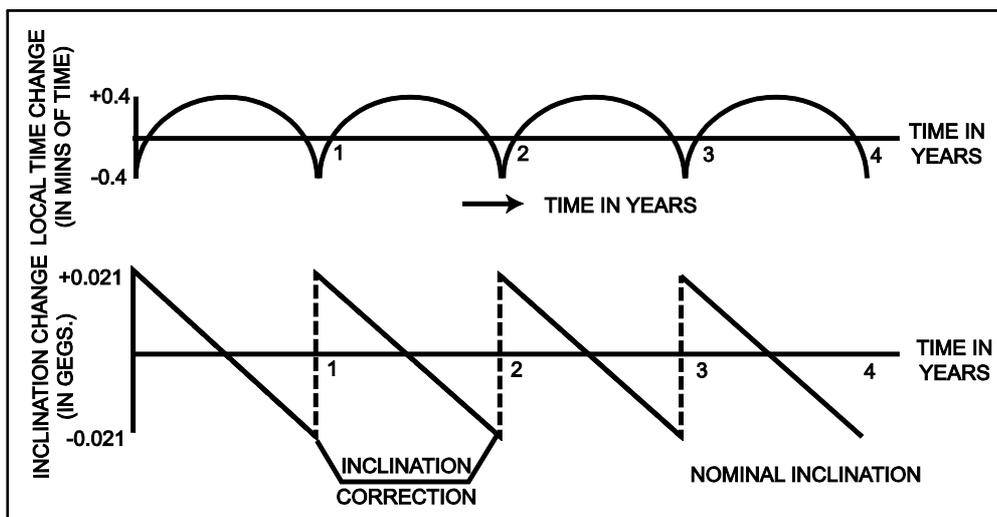
Figure 3.11 Local time control by inclination correction
