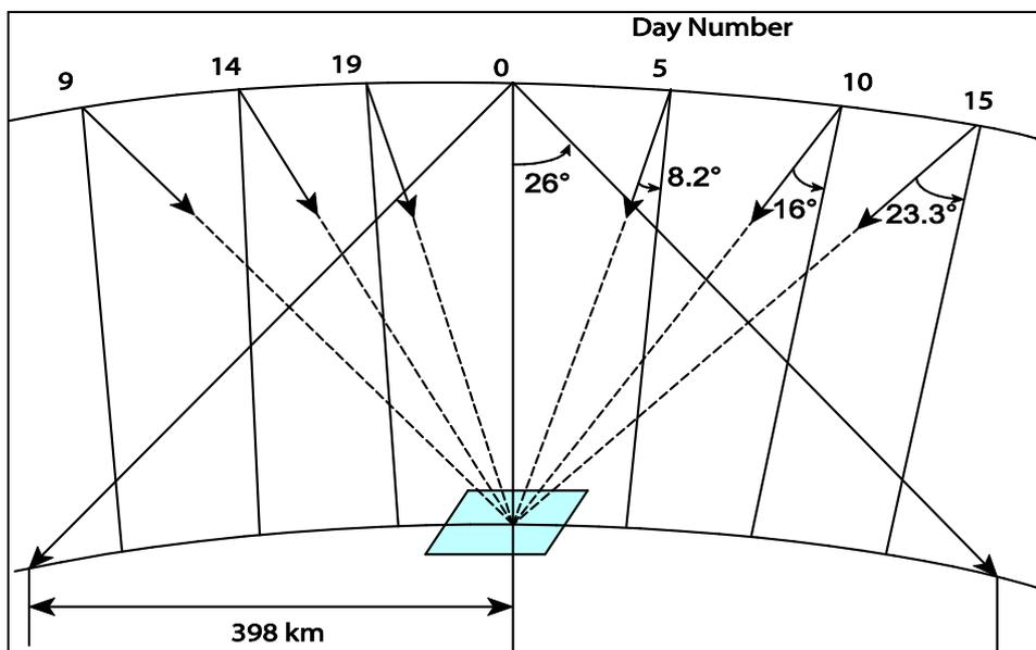
Figure 3.3 Coverage due to LISS-IV off-nadir capability
