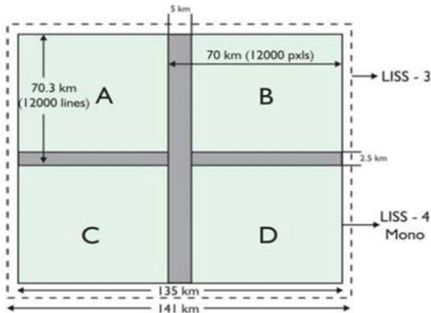
**Figure 3.6 LISS-IV scene (Mono) within a LISS-3 scene**
