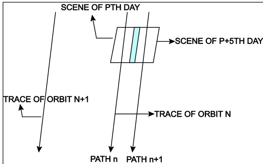
Figure 3.4 LISS-III coverage pattern.
