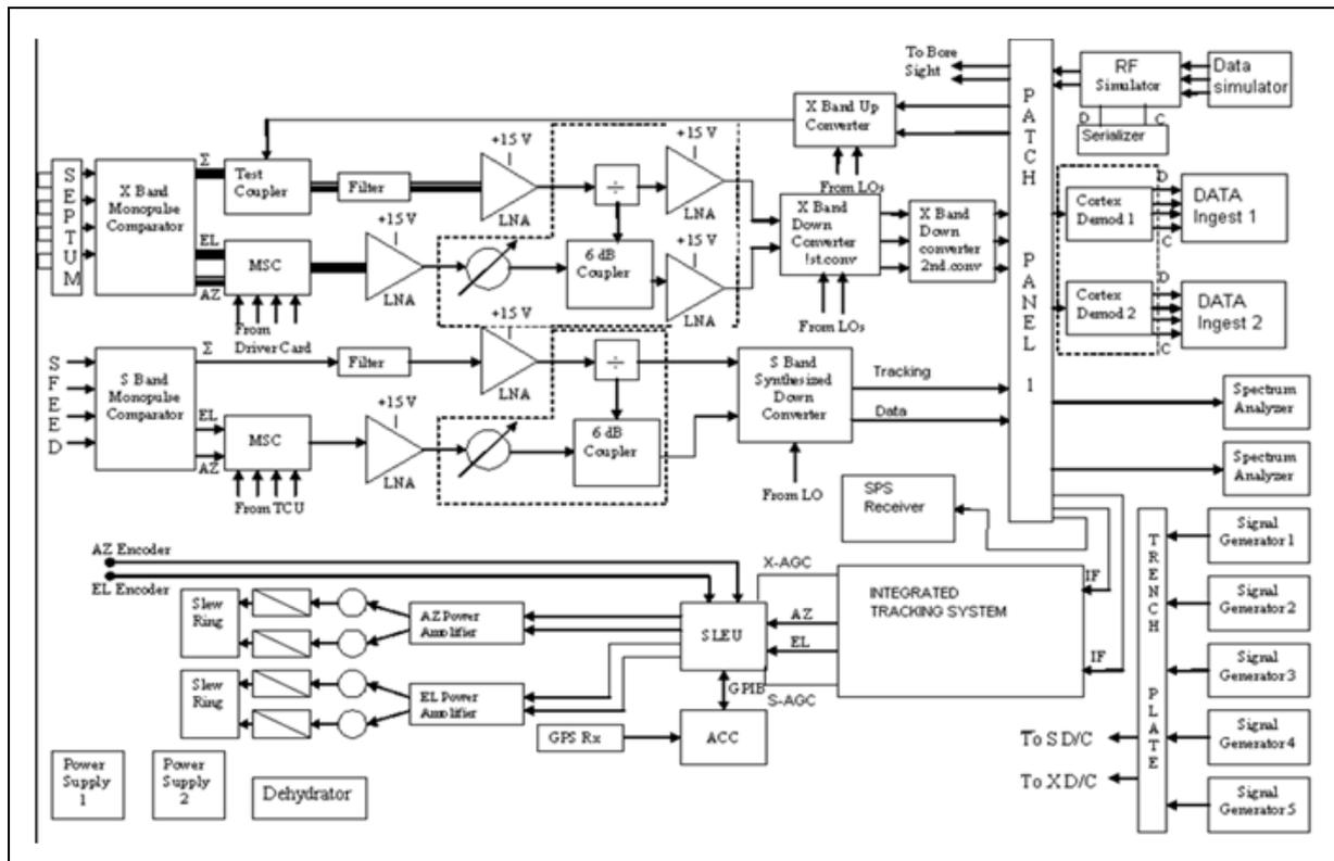
Fig. 5.6 Block Schematic of Data Receive system
