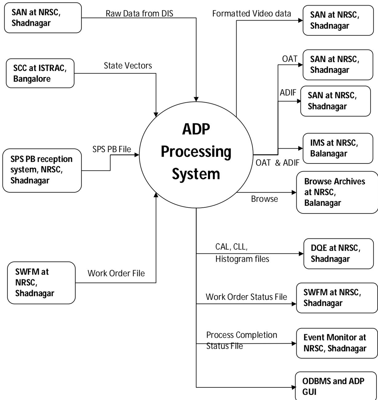
Fig. 6.5 Overview of ADP Processing System
