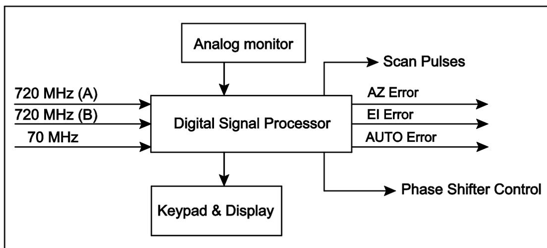
Fig. 5.3 Block Diagram of Integrated Tracking Systems (ITS)
