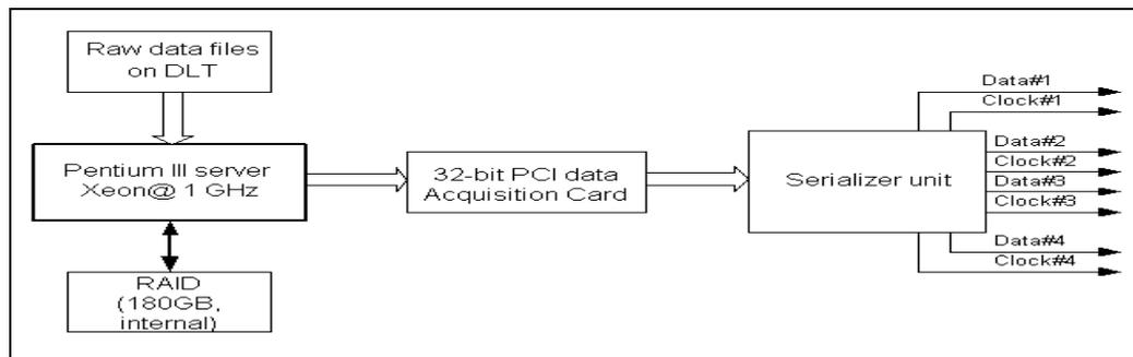
Fig. 5.14 Functional Block diagram of data serializer system
